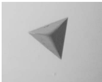
Figure 1 A crystal of recombinant HtrA protease domain. Crystal dimensions are about 0.3 \times 0.3 \times 0.2 mm.
